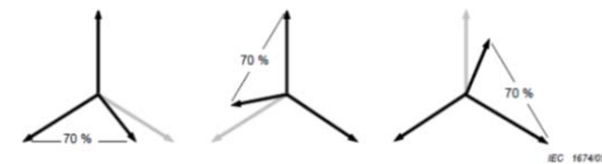
Figure 3b – Phase-to-phase testing on three-phase systems – Acceptable Method 1 phase shift
