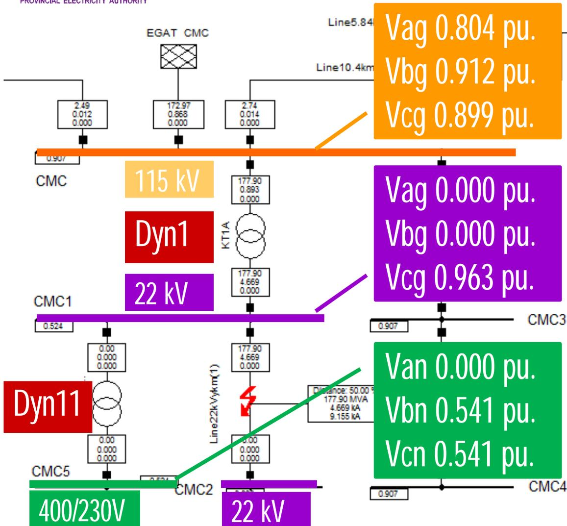
Double line to ground Fault
