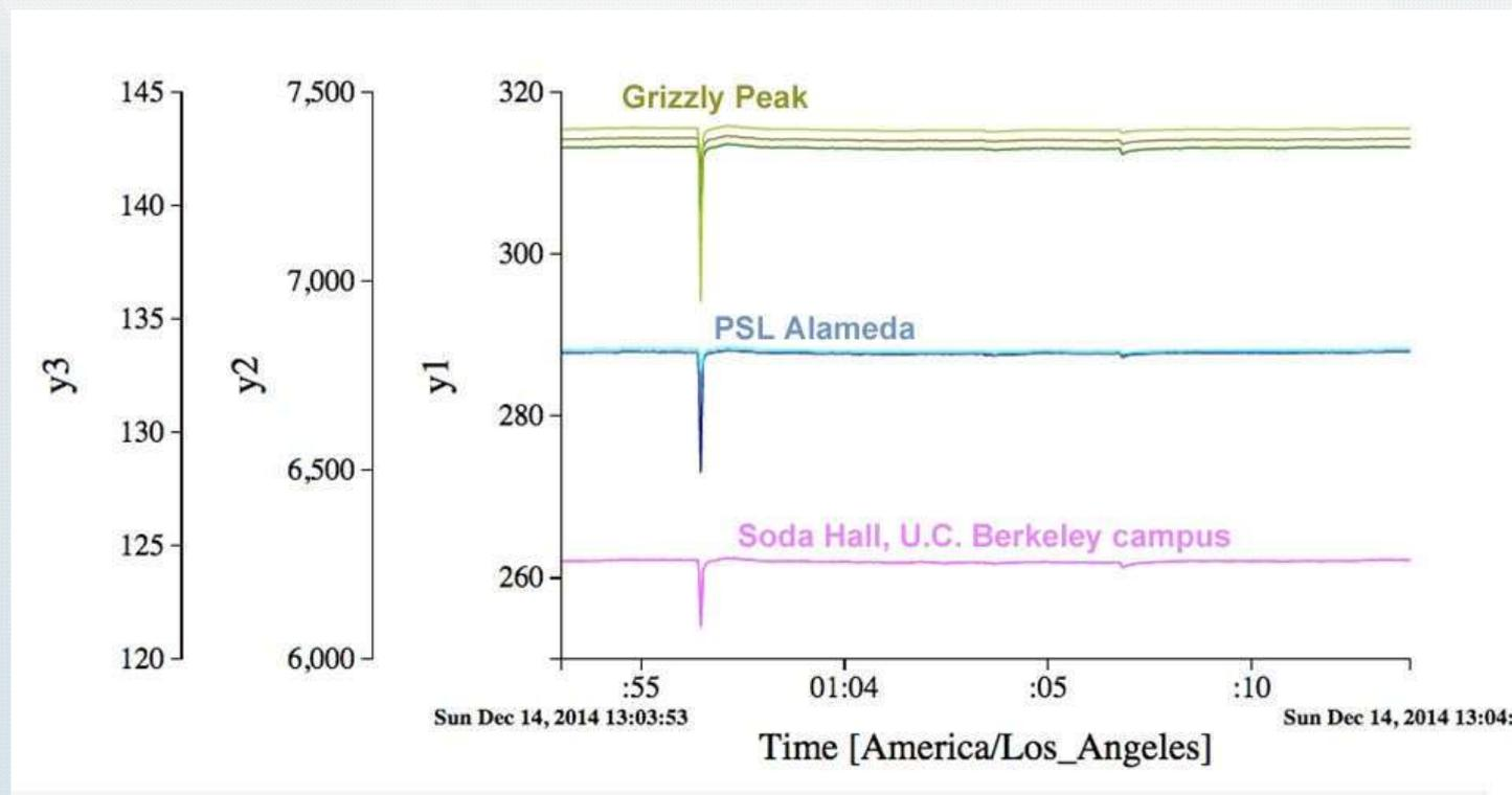
Simultaneous sags, at many locations: must be a transmission-level sag.
