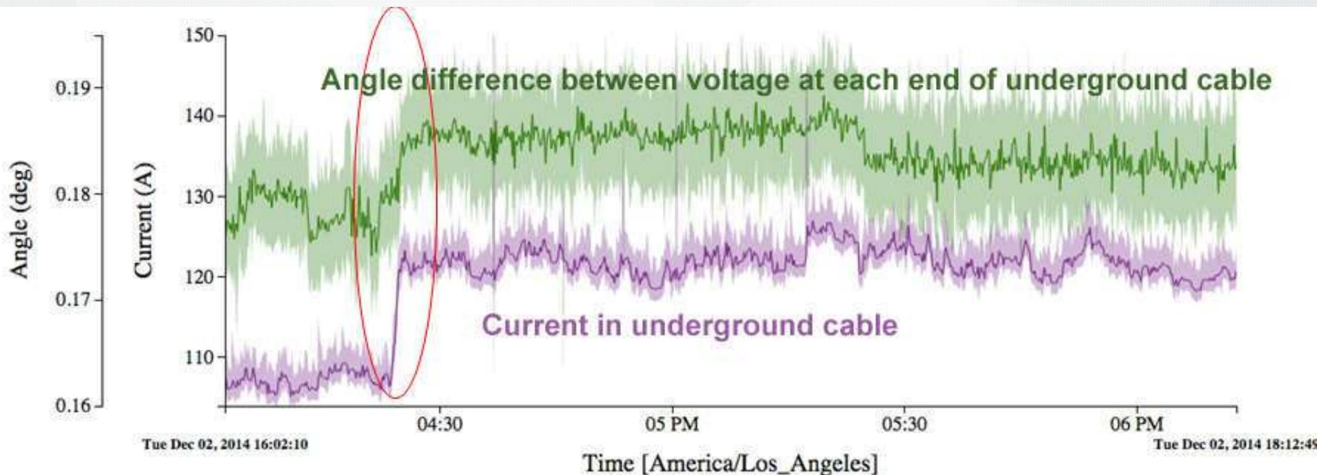
An increase in current causes a voltage phase angle change of  $0.008^\circ$  - typical resolution of the microPMU.
