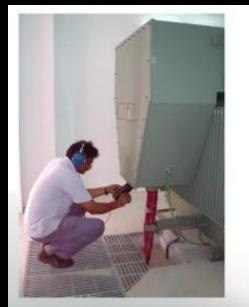
Acoustic Partial Discharge detection
