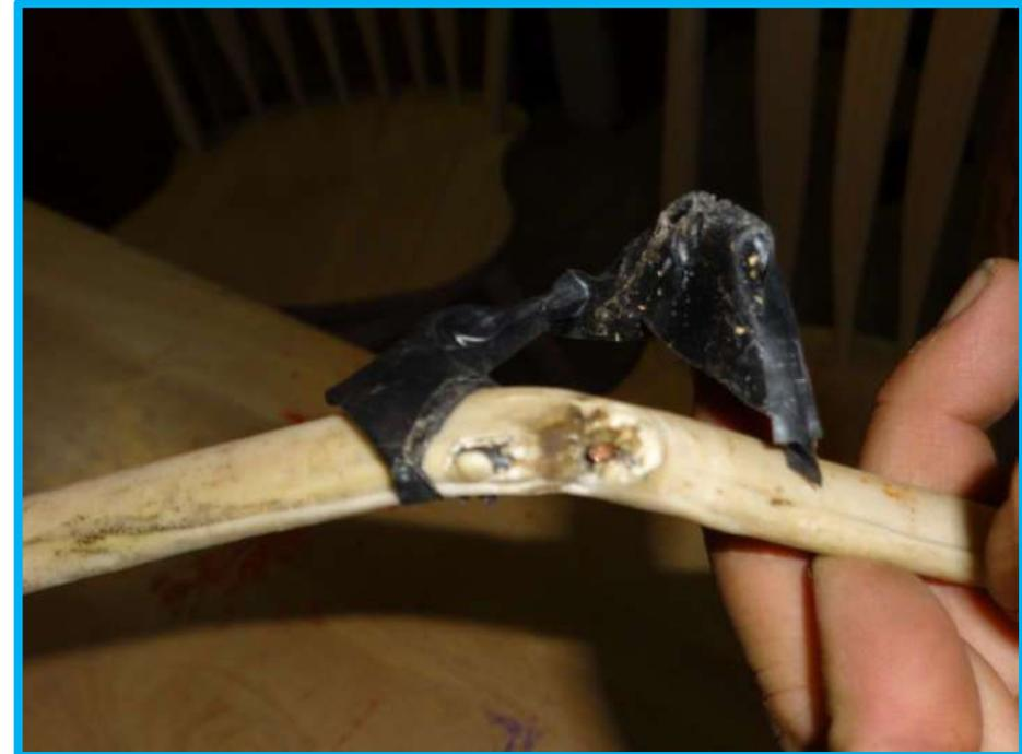
Wire damaged during construction/maintenance
