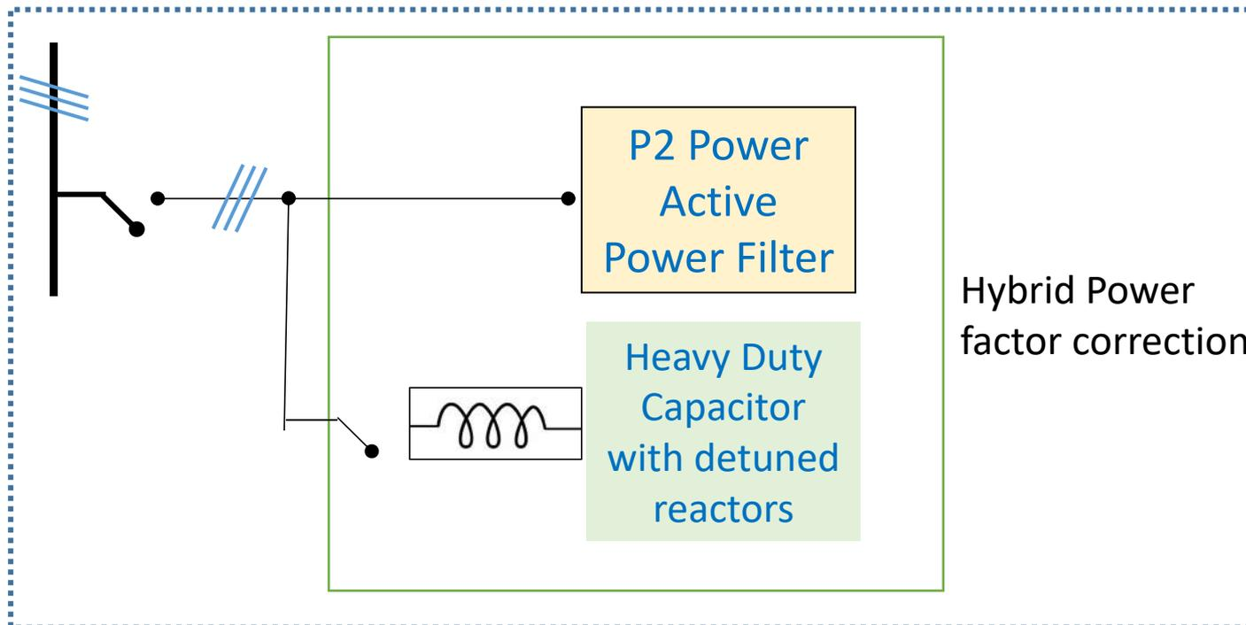
Hybrid PFC has an Active Power Filter along with heavy duty APP type detuned capacitor banks
