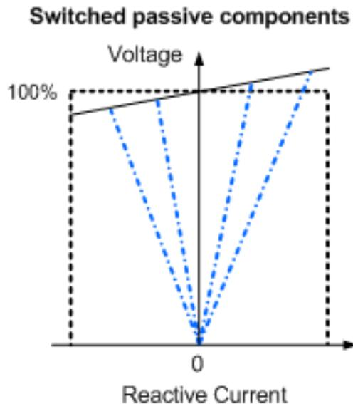
The simplest solution is without any doubts a combination of switched passive elements, i.e. switched capacitors and inductors.
