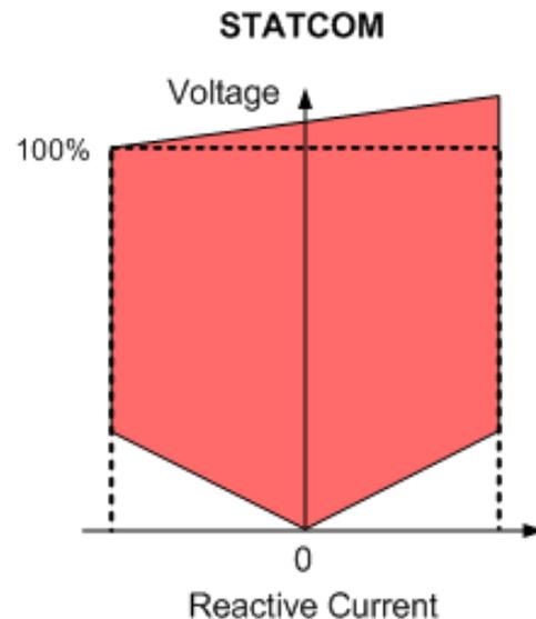
Figure to the left shows the reactive current versus connected voltage of a STATCOM. The performance is similar to a SVC, i.e. it performs smooth variation of reactive current across its operating range with high dynamics. It has some advantages when compared to the Static Var Compensator (SVC), e.g., current injection independent of the system voltage, faster control and less of a space requirement.
