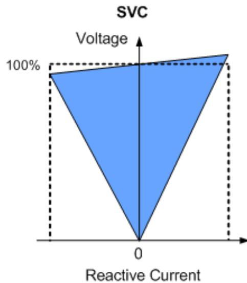
Figure to the left shows the reactive current versus connected voltage of a widely used reactive power compensator: the SVC (Static VAr Compensator). The SVC combines thyristor switched capacitors (TSC) with thyristor controlled reactors (TCR). Doing so, a smooth variation of reactive power over the complete installed power range is possible.
