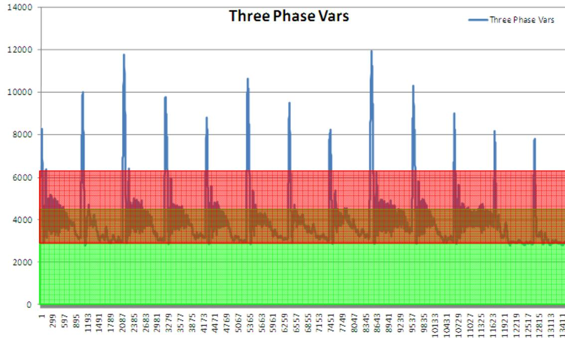
Figure 7: Variation in reactive power during shredding cycle
