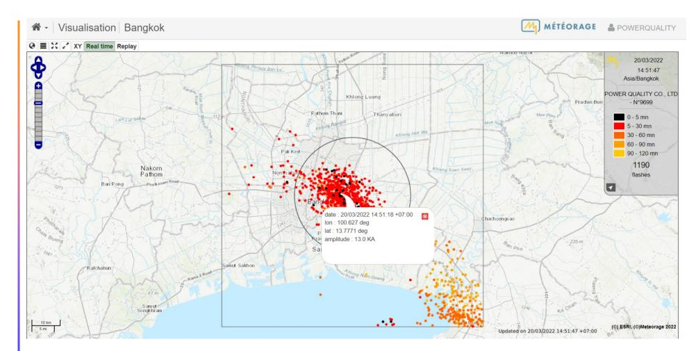
Selecting each lighting point detected on the map will provide further details as shown on the image. \*The color code shows the chronology of strikes on the map.
