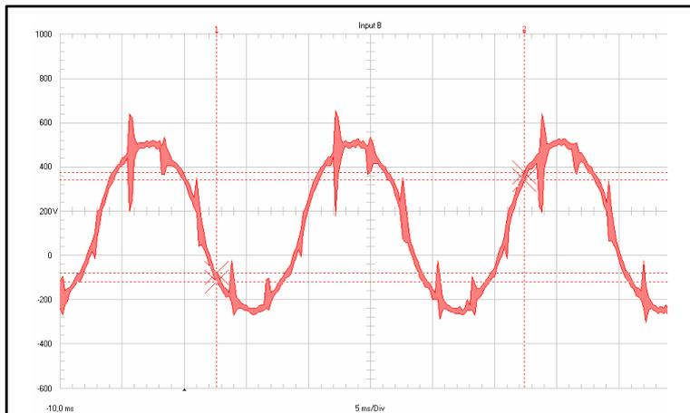
*Figure 2: Voltage waveform at input to harmonic filter*
