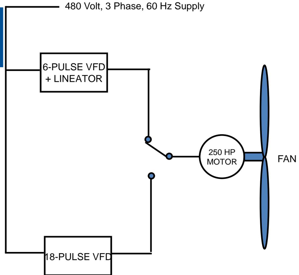
**6-PULSE DRIVE + LINEATOR saved 3.5% to 6% of energy needed to run fan**
