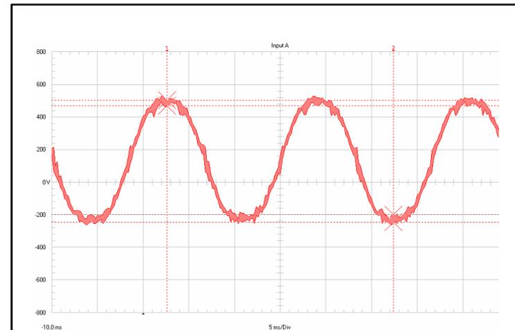
*Figure 3: Voltage waveform at output of harmonic filter supplying AC Drive*
