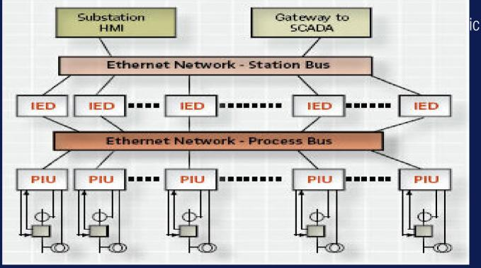
Station bus Ethernet for <u>Human Machine Interface (HMI)</u> to <u>Intelligent Electronic Device (IED)</u>
