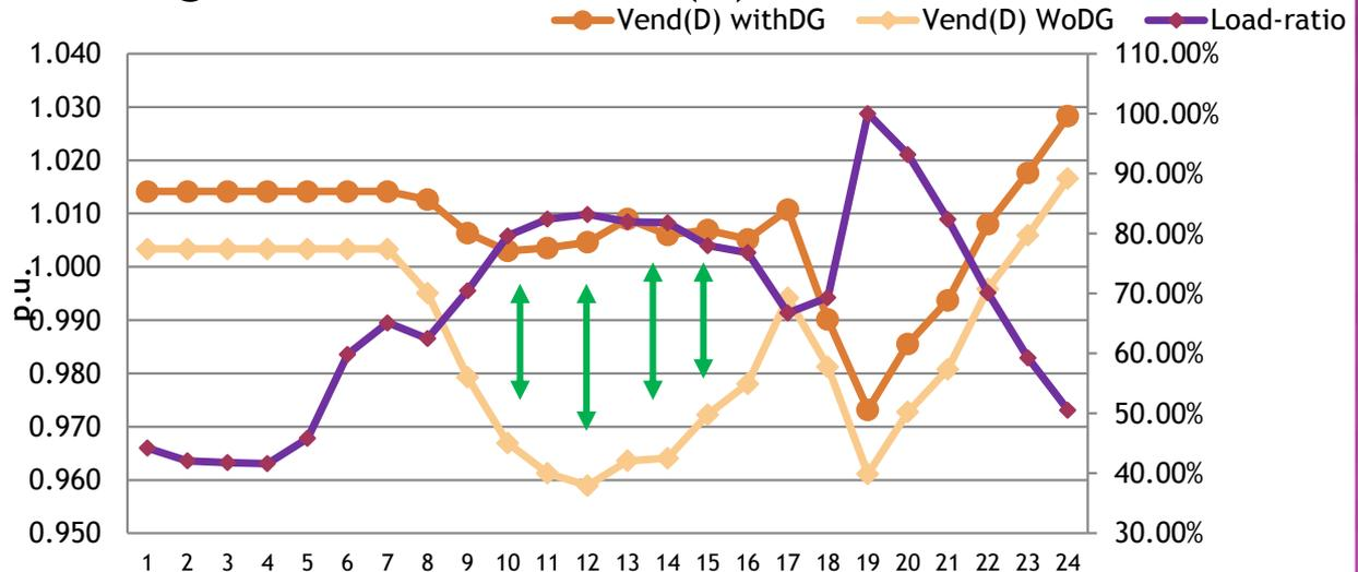
Figure 9 Result of voltage profile 24 hrs. at Endline (D)
