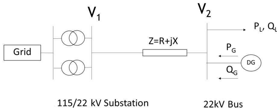
Normally, before allowing the installation of DG, the Distribution System Operation will ensure that the voltage, line thermal characteristics and substation transformer capacity will not be violated for the worst operating scenarios:
