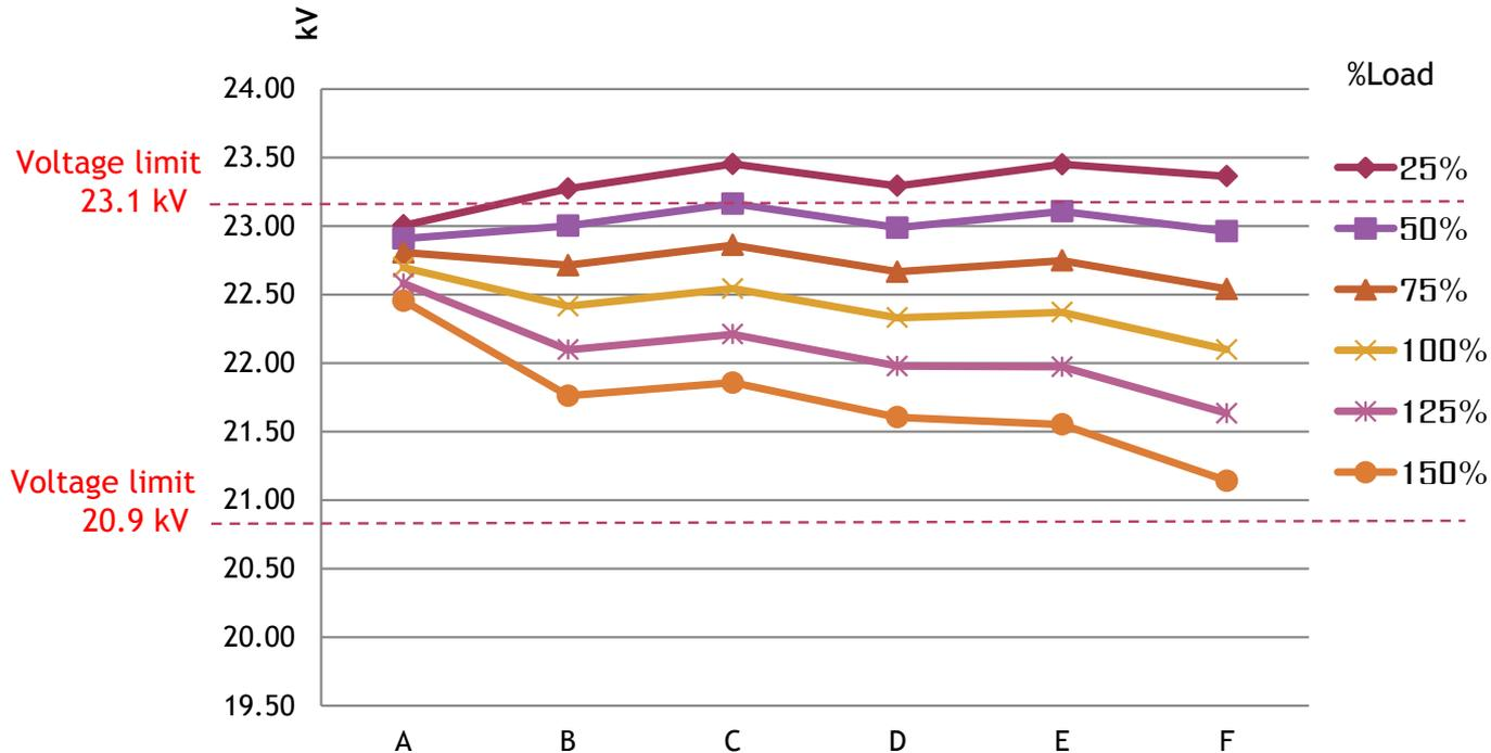
Figure 11 Result of voltage level with vary of load from 25% - 150%
