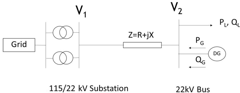
Figure 1 Illustration of a DN with DG connected
