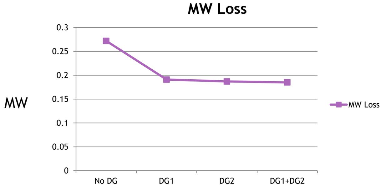
Figure 14 Result of Power Loss with vary of DG installation rating
