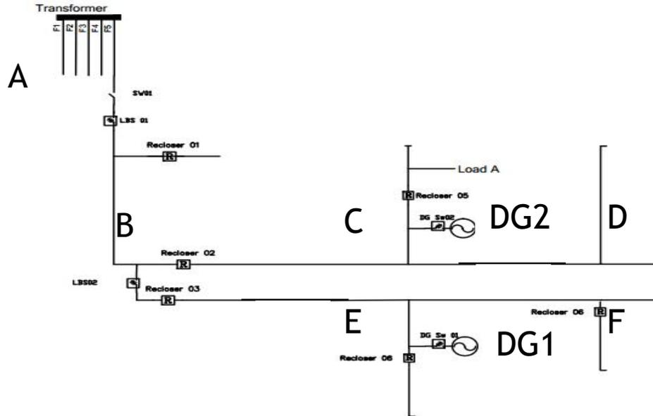
Figure 4 Radial DN 22 kV of PEA in the northeast area of Thailand
