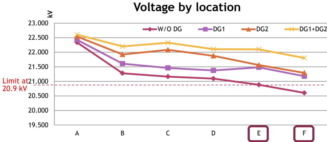
Figure 10 Result of voltage level at each location
