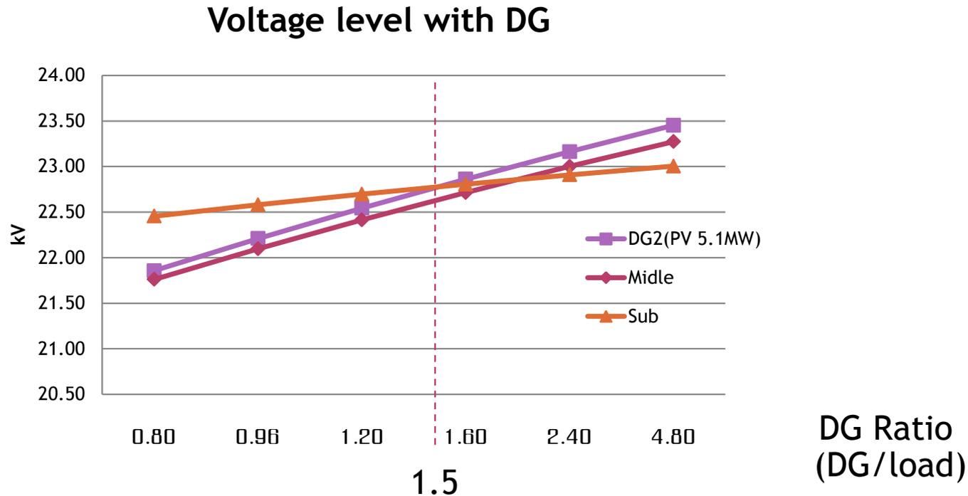
Figure 13 Result of voltage level with vary of DG Ratio
