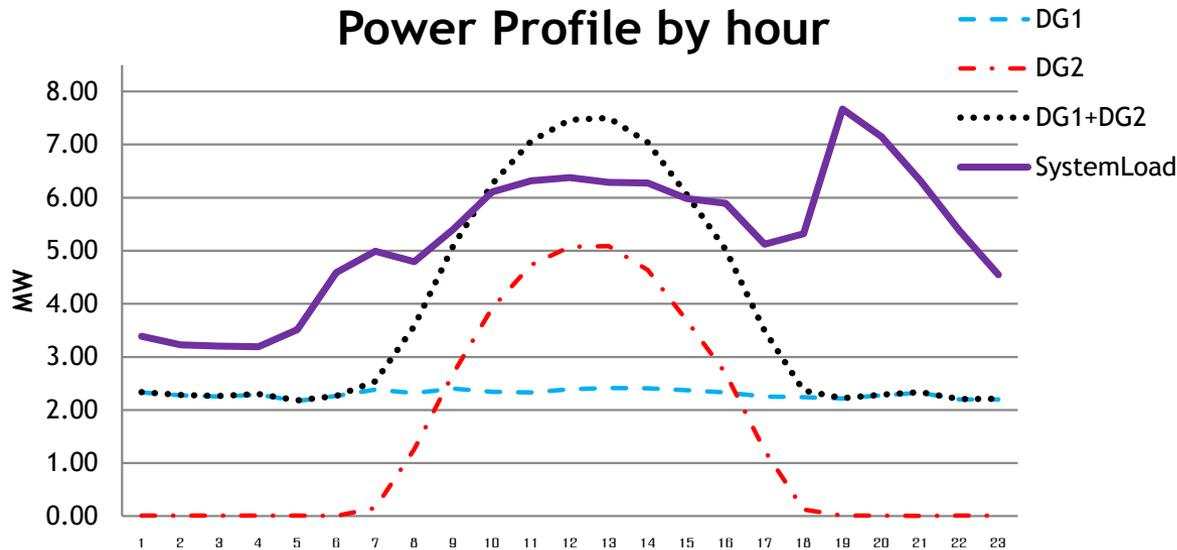
Figure 5 Power Profile of load and DG generation rating 24 hrs.
