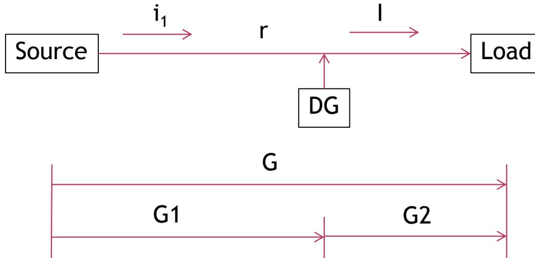
Figure 4 Simple model of Distribution system with DG installation
