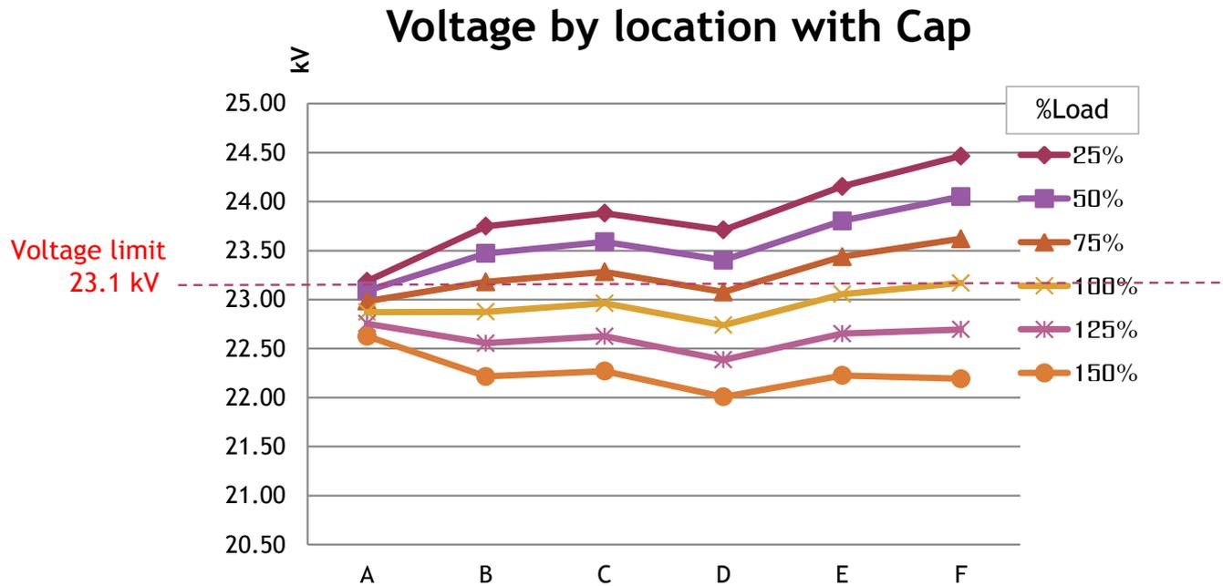
Figure 12 Result of voltage level with vary of load from 25% - 150% with support of switching capacitor installation.
