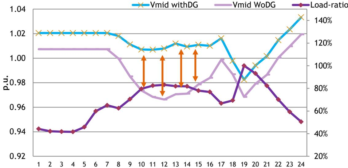
Figure 8 Result of voltage profile 24 hrs. at Midline (B)
