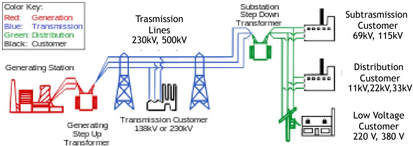
The power flow is in one direction only, from the transmission system to the HV substations and to the MV&LV distribution system.
