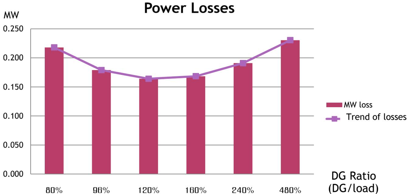
Figure 15 Result of Power Loss with vary of DG Ratio
