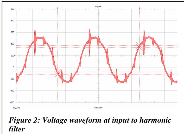
Voltage Notching Caused by DC Drives on Off-shore Oil Platform
