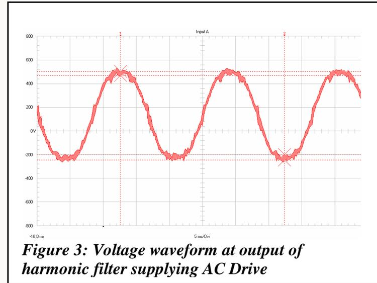
Notches Dramatically reduced on Output of Lineator AUHF
