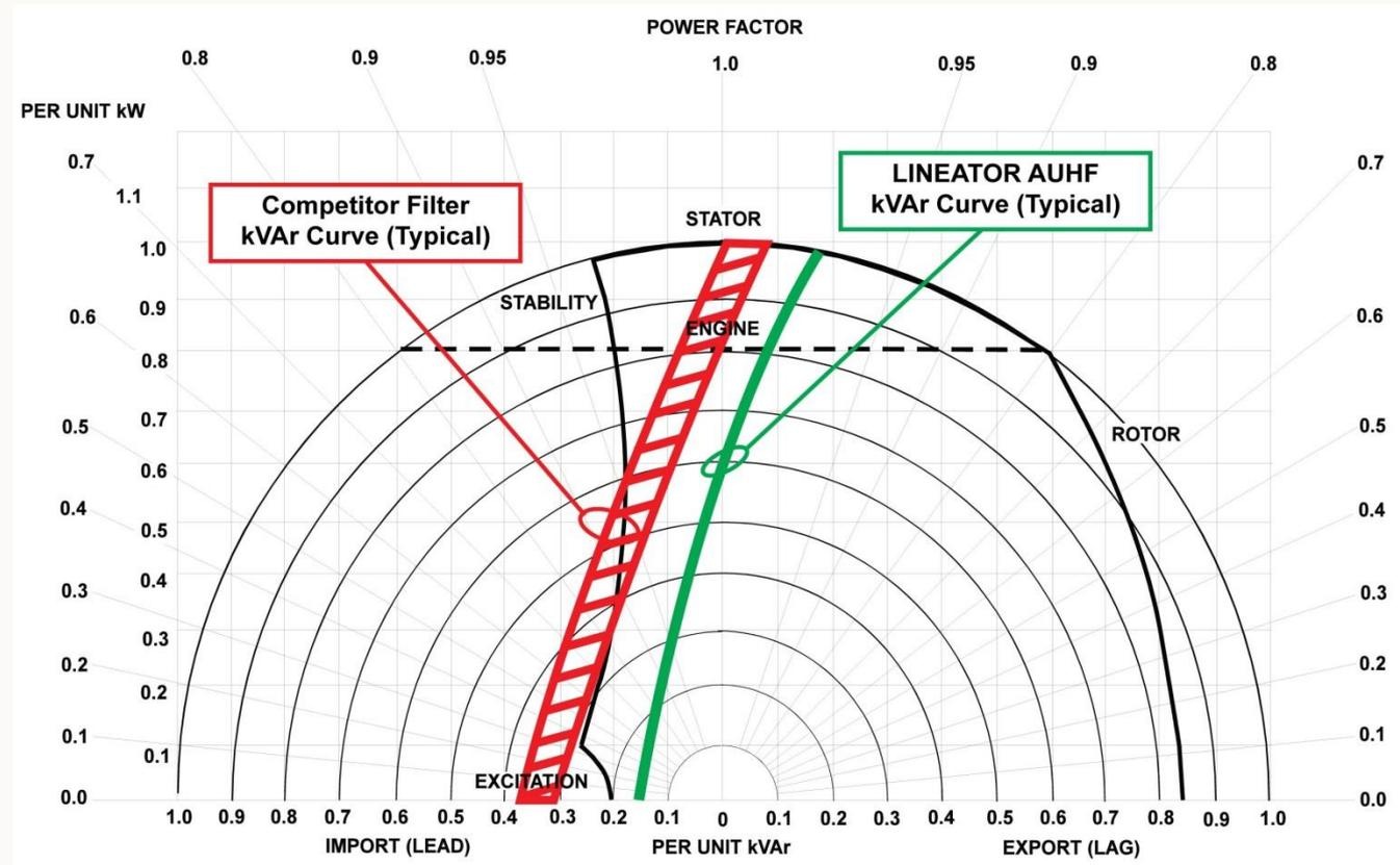
Maximum Capacitive Reactance introduced by Filter ———
