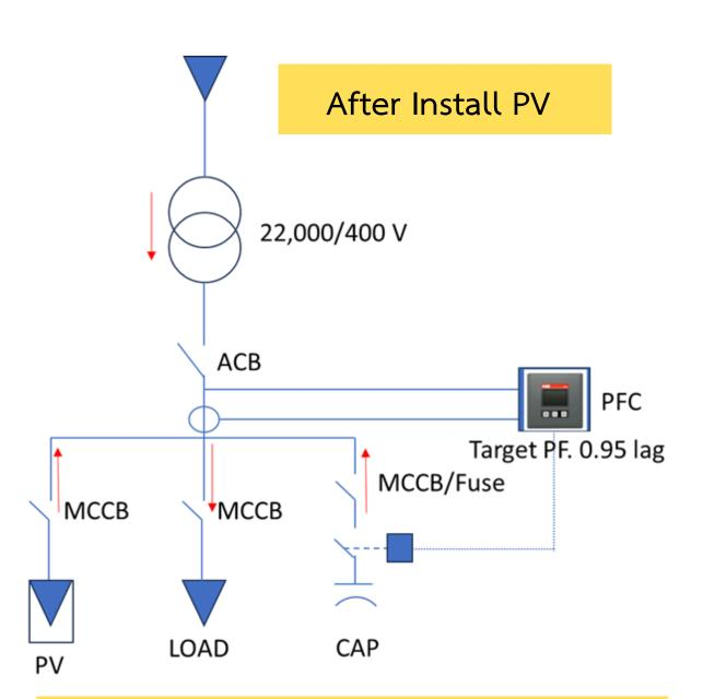
Active Power From grid trought CT But Active Power From PV direct to load.
