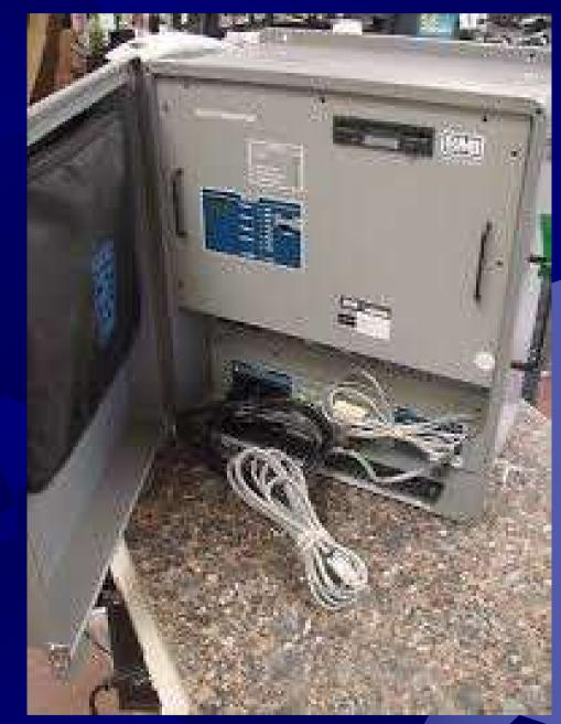
1990's RPM All Digital recorders 4 voltage, 5 current all **10** PQ parameters Every cycle all channels gapless maximum time years All power parameters Network connection and database Software becomes more important Market disruption with all digital no UI, no setup, every cycle all the time
