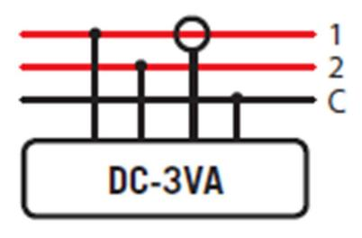
Two DC voltage channels; 300Vdc One DC current channel; bidirectional 10/100Adc
