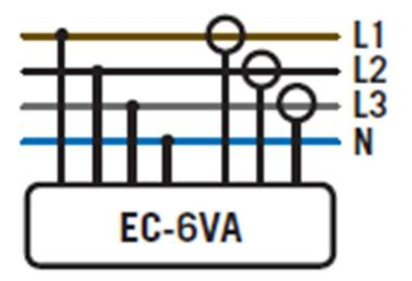
Three voltage channels 500Vac Three current channels 400A, 1kA, 2kA or 3kAac
