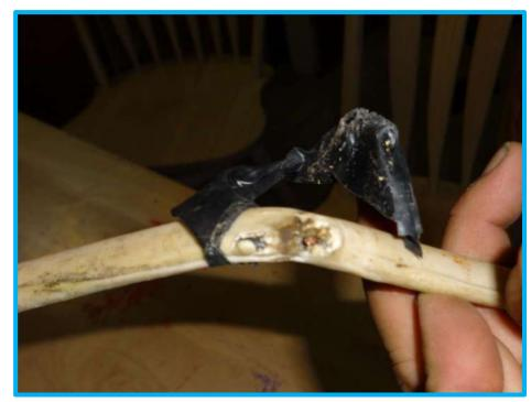
Wire damaged during construction/maintenance
