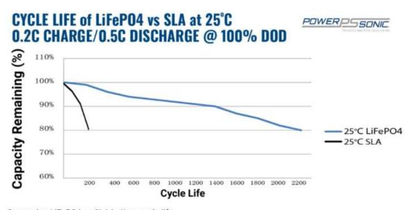
Comparing LiFePO4 vs SLA battery cycle life
