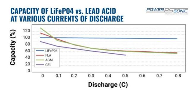
Capacity of lithium battery vs different types of lead acid batteries at various discharge currents
