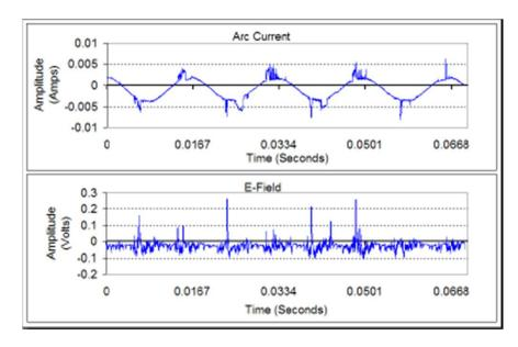
**Current profile for a Neon Sign can include transients**
