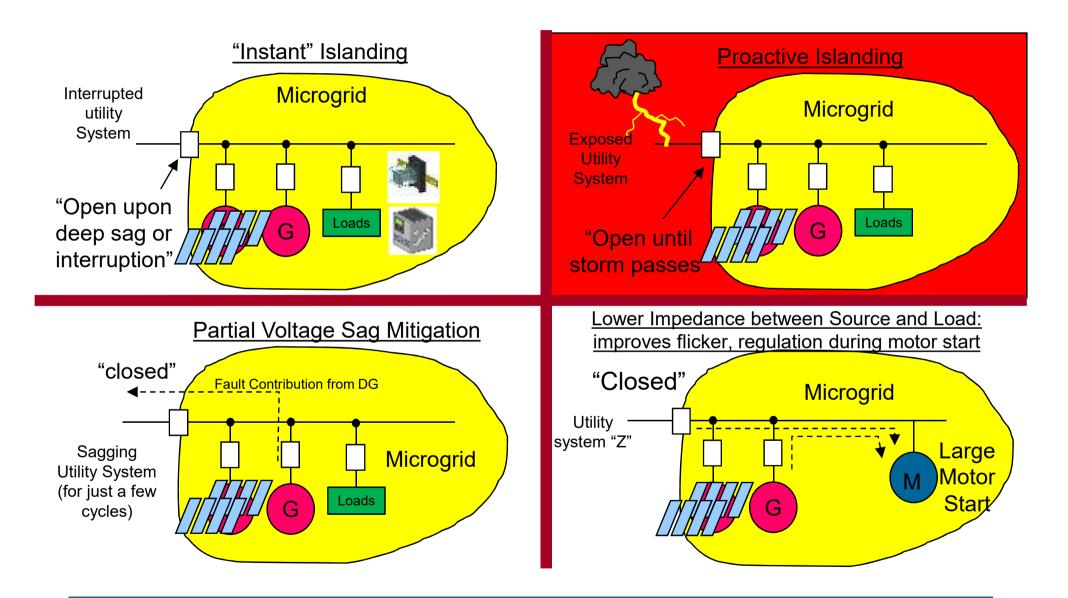
All of our regular PQ standards are for grid-connected systems. We haven't really even begun to develop comparable standards for transitioning to local, islanded generation
