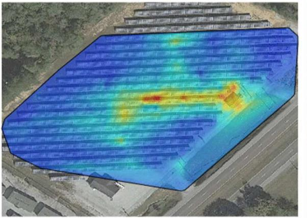
Radiated Emissions from this PV Installation:
