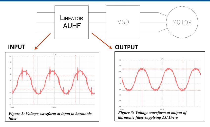
Voltage Notching Caused by DC Drives on Off-shore Oil Platform
