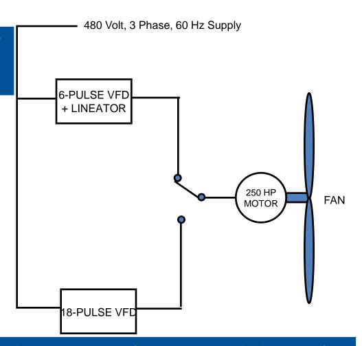
6-PULSE DRIVE + LINEATOR saved 3.5% to 6% of energy needed to run fan
