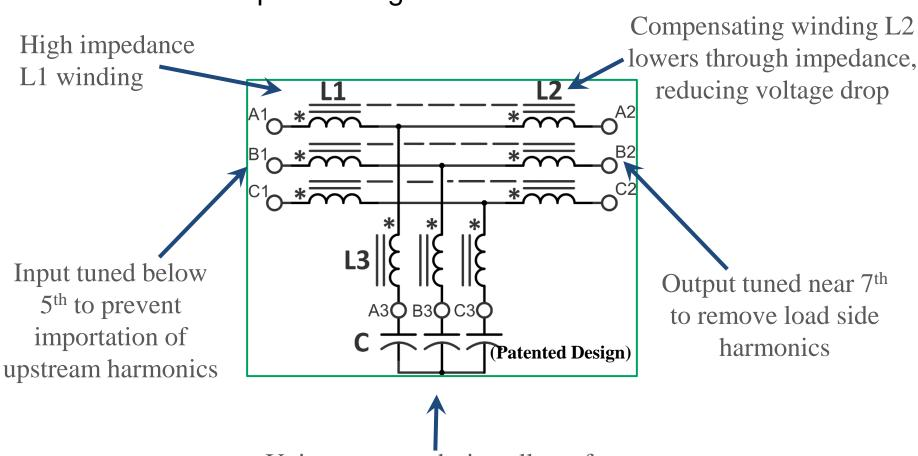
Unique reactor design allows for smaller cap bank to reduce voltage © 2015 Mirus International | All Rights Reserved boost and reactive power at no load
