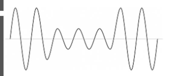
IEC STANDARDS REQUIRES A LENGTH OF 10 CYCLES TO BE CAPTURED, ALLOWING HARMONICS TO BE CALCULATED. SOME PQ METER DESIGNS MAY HAVE DIFFICULTY IN CORRECTLY RECORDING THE 11 CYCLE EVENT ACCURATELY.
