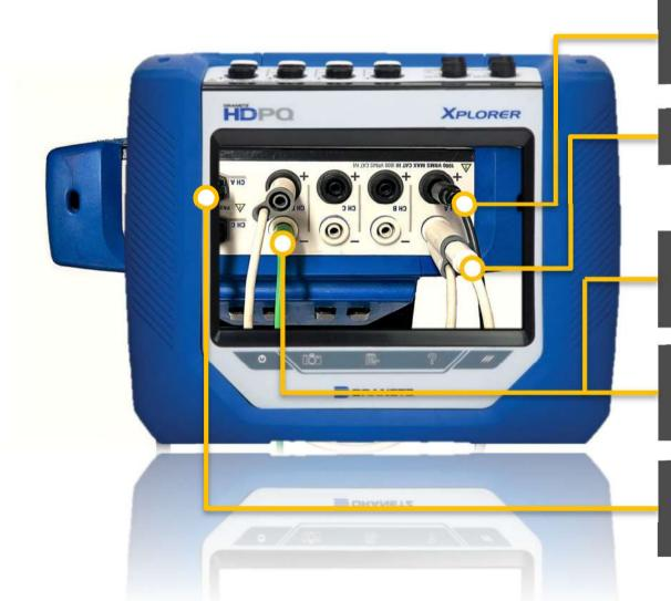
OUTPUT PHASE VOLTAGE TO THE PQ METER VOLTAGE CHANNEL PHASE A +
