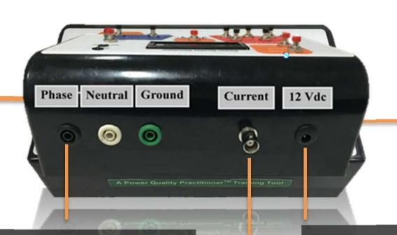
OUTPUT PHASE VOLTAGE 120 ~ 240 VAC, 50-60Hz
