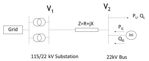
Figure 1 Illustration of a DN with DG connected
