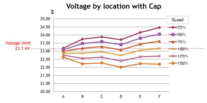
Figure 12 Result of voltage level with vary of load from 25% - 150% with support of switching capacitor installation.
