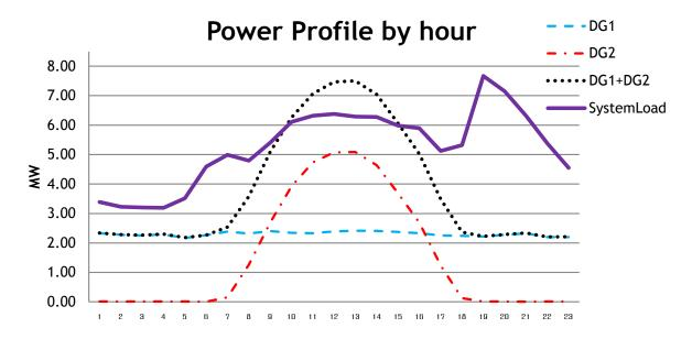
Figure 5 Power Profile of load and DG generation rating 24 hrs. DG1 Biomass-based: generate power at 2.4 MW average DG2 PV: generate power only day time vary by sunrise cycle, max at 5.1 MW System load: dispersed along line, most are residential consumers. Commercial & Business consumers: sugar factory and small business. Peak load at night time(07.00-09.00 pm.) By day time total load was lower than the generation of DGs.
