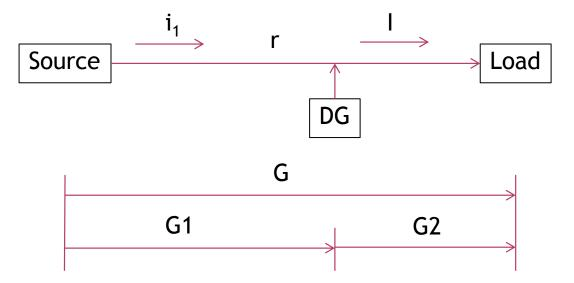
Figure 4 Simple model of Distribution system with DG installation
