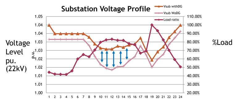
Figure 7 Result of voltage profile 24 hrs. at Substation
