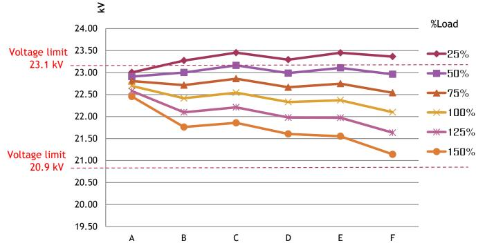
Figure 11 Result of voltage level with vary of load from 25% - 150%
