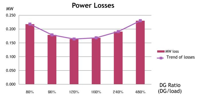
Figure 15 Result of Power Loss with vary of DG Ratio
