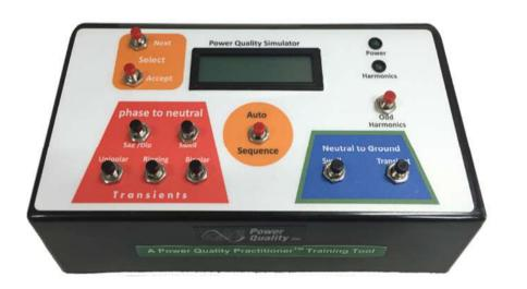
• Firstly, connect PQSim to Power Quality Meter and then configure it for capturing harmonics.
